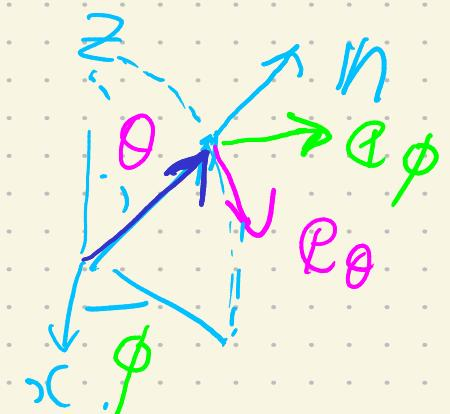
$$\frac{\delta\theta}{\delta S} = \frac{1}{S}(\cos\theta\omega\phi, \omega\sin\theta\sin\phi, -\sin\theta) = \frac{1}{S}\Phi_\theta$$
