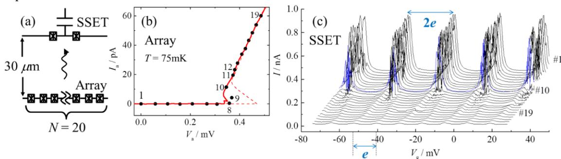
Figure 1: Coulomb oscillations of the SSET with their  $2e$  periodicity modulated to  $e$  by the bias voltage of the remote array. Inter-device distance was  $30\ \mu\text{m}$ . The measurement temperature was 75 mK. (a) schematic device arrangement. (b)  $I_a$ – $V_a$  characteristics of the array. (c)  $2e$  to  $e$  modulation of the Coulomb oscillations of the SSET. References
