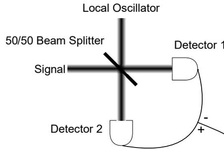
Figure 1: Schematic figure of optical balanced homodyne detection. After the signal mode is mixed with the local oscillator by a 50/50 beam splitter, the two output modes are detected by two different photodetectors. The difference in detected photon number is recorded.
